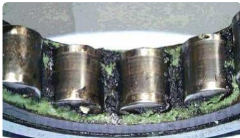
Lubricant degradation caused by electrical discharge currents
