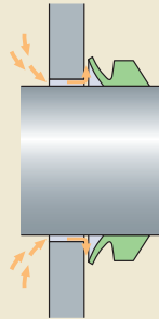
V-ring used as a grease valve
