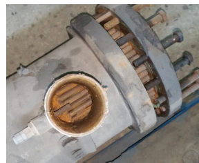
Disconnect to see tube diameter and pitch
